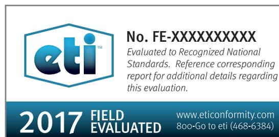
**Figure 1.** One of the most common forms of evidence considered acceptable by AHJs is the labeling by a third party.
